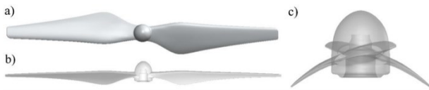
Figure 3 DJI Phantom Propeller a) Top view; b) Front view; c) Side view
