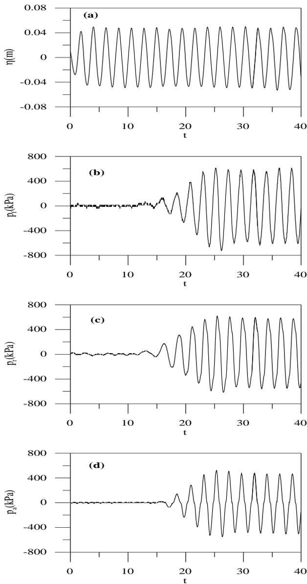
**Figure 3** Time history of (a) incident wave surface elevation (b) front wall pressure (c) rear wall pressure and (d) air pressure
