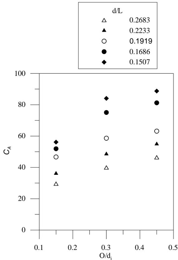
**Figure 5** Effect of relative bottom opening on wave power absorption efficiency
