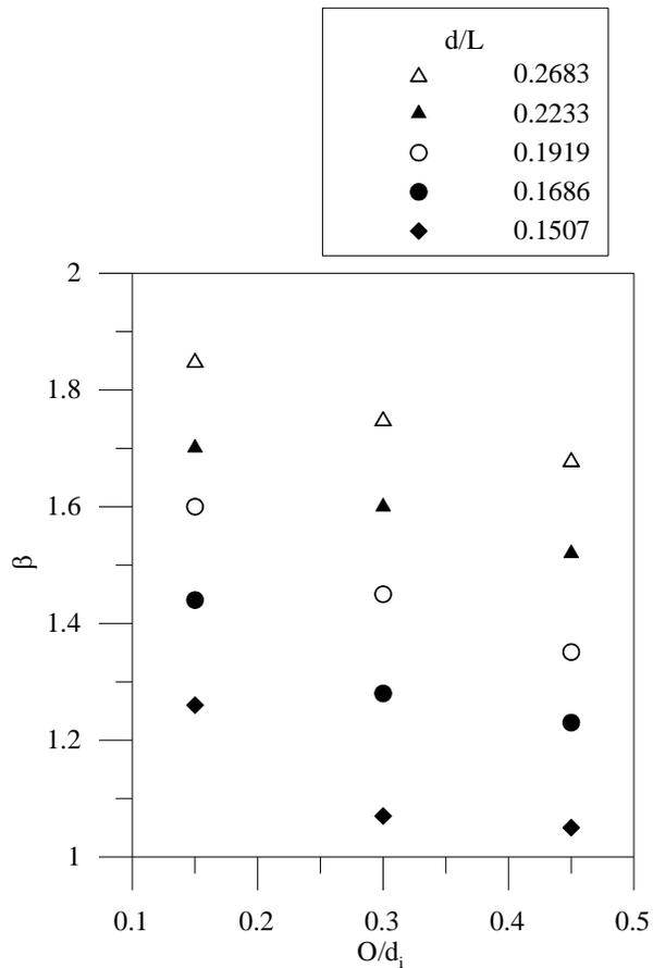
Figure 7 Effect of relative bottom opening on wave amplification
