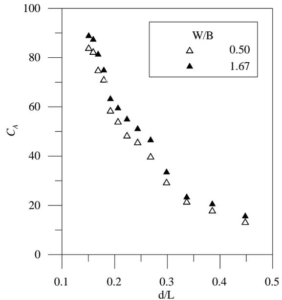
**Figure 4** Effect of water plane area on the variation of  $C_A$  with  $d/L$
