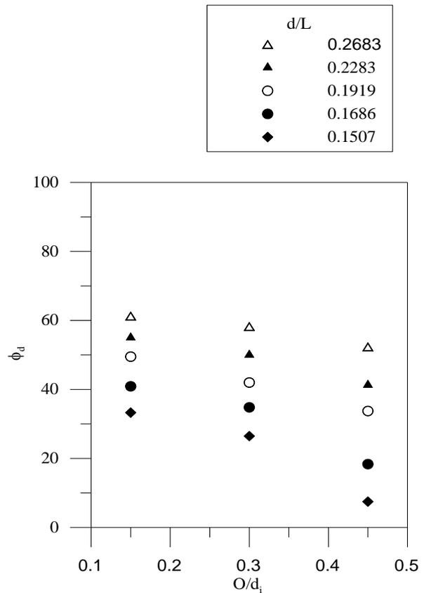
**Figure 6** Effect of relative bottom opening on phase angle variation
