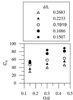
Effect of relative bottom opening on wave power absorption efficiency
