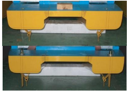
Figure 4 Rear views of ship models with three different hull clearances (top: S, middle: M, bottom: L)
