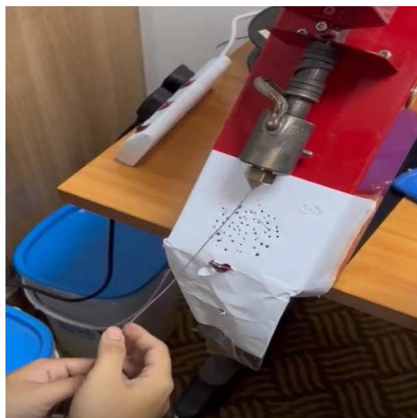
Figure 1 The extrusion process of PET-GNPs filament using mechanical extruder machine
