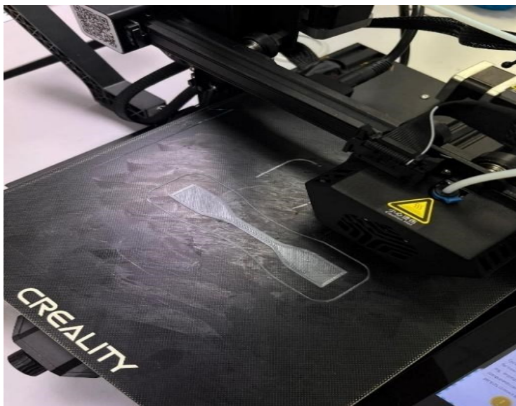
Figure 2 Creality 3D-printer machine used to 3D print dog bone and square shape for tensile test and gas permeability characterization
