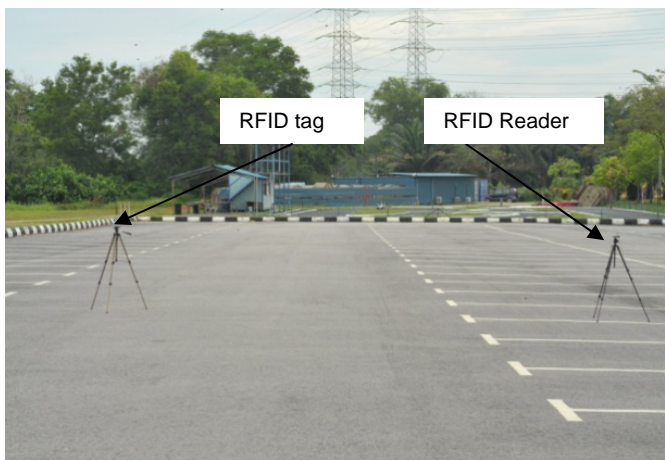
Figure 7 Measurement setup at Padang Kawad (Open Space)
