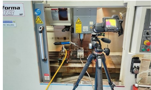
Figure 3 Thermal camera setup
