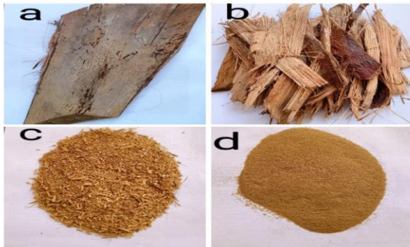
Figure 2 Stages of grinding date palm fiber material
