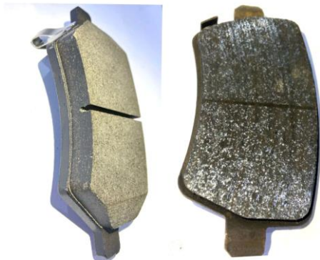
The change in brake pad shape due to thermal overload.
