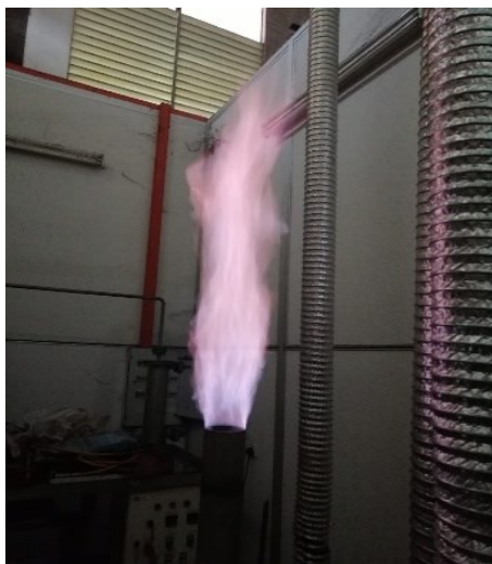
Figure 3 Flare flame observation for 16 m 3 /h airflow rate
