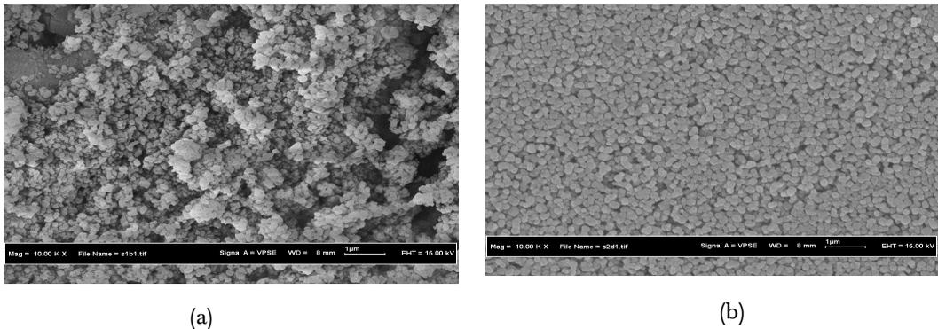
**Figure 5** FESEM micrographs of (a) TiO<sub>2</sub> immobilized on cement (b) TiO<sub>2</sub> immobilized on tile
