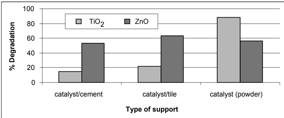
**Figure 4** Comparison of catalyst efficiency for TiO<sub>2</sub> and ZnO catalyst, without and using cement and tile as support over degradation of paraquat using UV light, 354 nm
