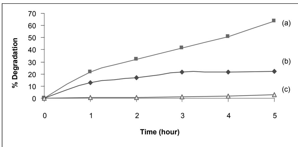
**Figure 2** Percentage degradation of paraquat for tile supported (a) ZnO, (b) TiO<sub>2</sub> and (c) tile after irradiation with UV light 354 nm
