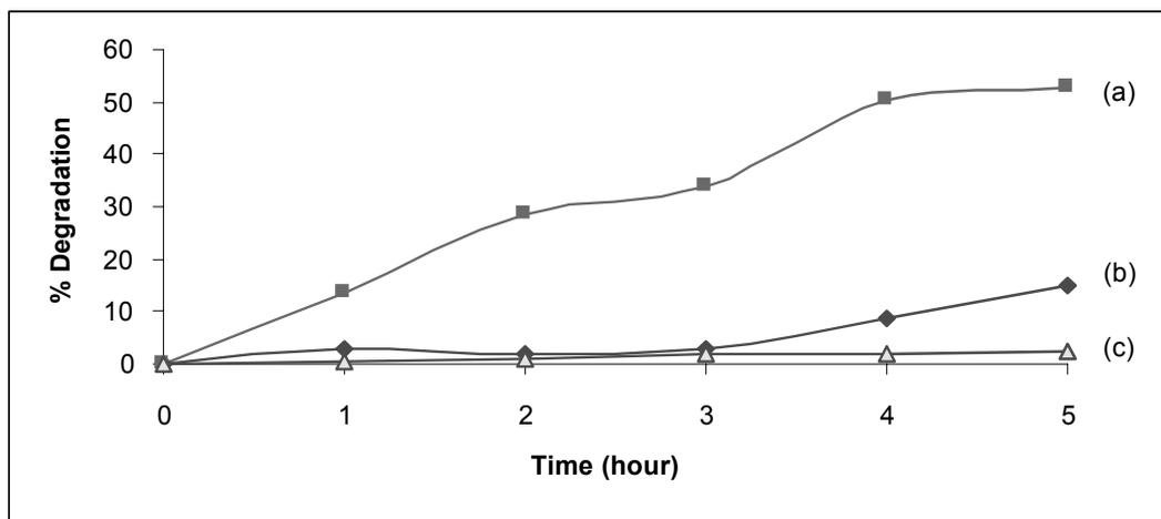
**Figure 1** Percentage degradation of paraquat for cement supported (a) ZnO, (b) TiO<sub>2</sub> and (c) cement after irradiation with UV light, 354 nm
