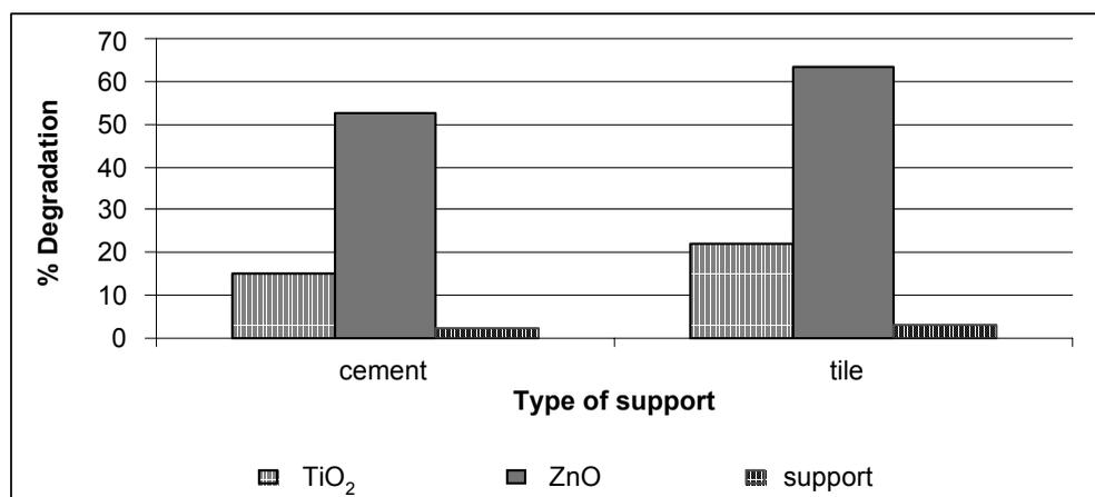
**Figure 3** Comparison of supports efficiency for supported TiO<sub>2</sub> and ZnO, over degradation of paraquat after 5 hours illumination using UV light, 354 nm
