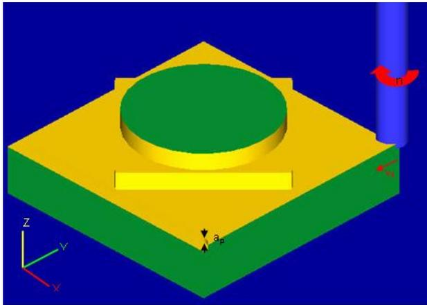
Figure 5 Layout of the outer square machining operation
