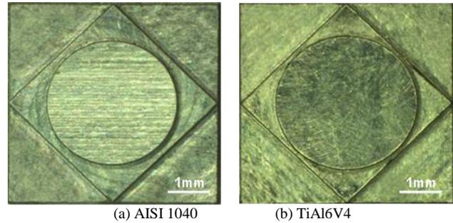
Figure 6 Machined micro-testpieces
