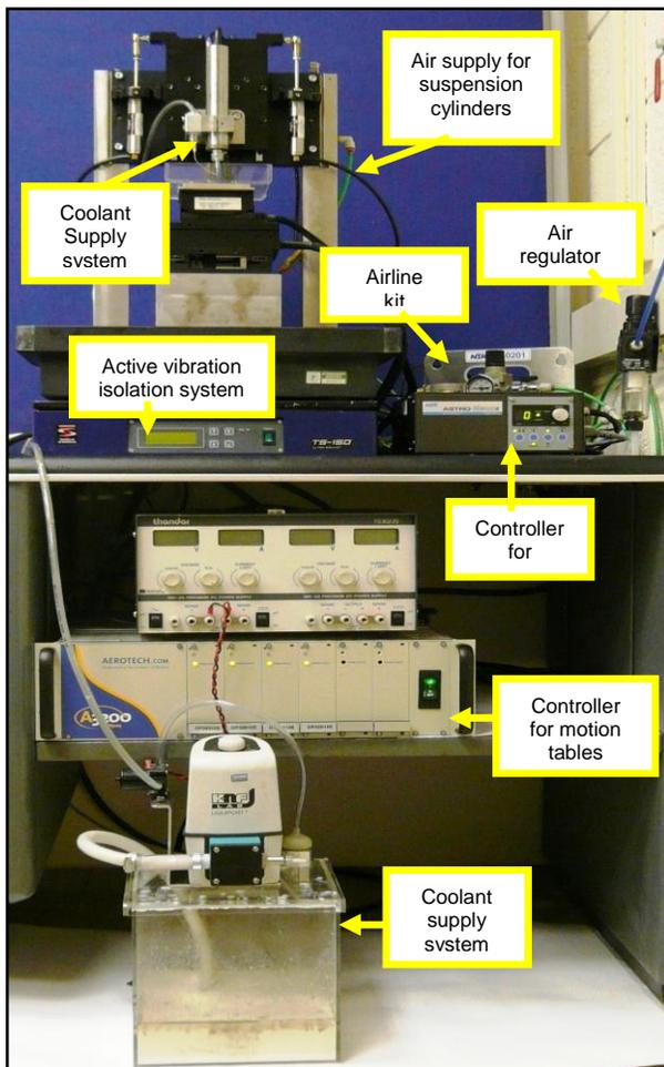
**Figure 1** The set-up of the miniature machine tool
