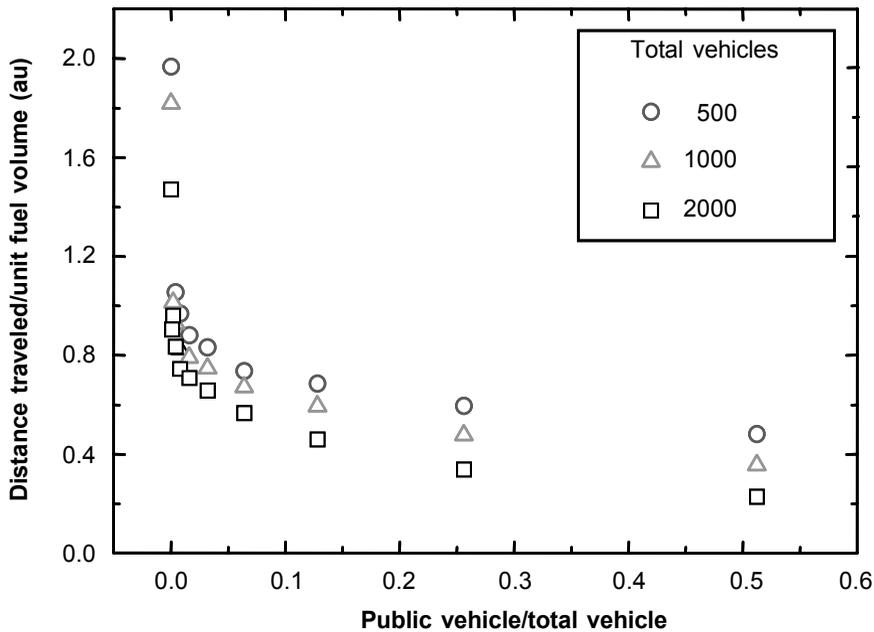
**Figure 6** Distance traveled per unit fuel volume as a function of ratio of public vehicles to total number of vehicles at different total number of vehicles (circle = 500, triangle = 1000, and square = 2000). The iteration step was fixed at  $10^4$ , the stopping time at 100 steps,  $p_c = 0.2$ , and  $\gamma = 0.1$
