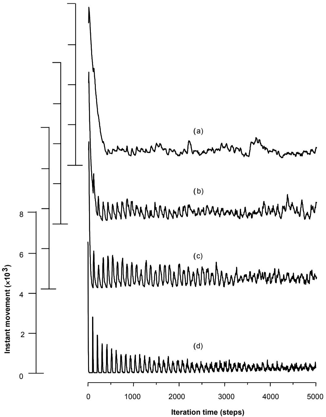
**Figure 3** Effect of iteration time on the instant total movement of all vehicles at different number of public vehicles [(a) = 10, (b) = 50, (c) = 100, and (d) = 500]. The total number of vehicles was fixed at 2000, the iteration step at  $10^4$ , the stopping time at 100 steps,  $p_c = 0.2$ , and  $\gamma = 0.1$
