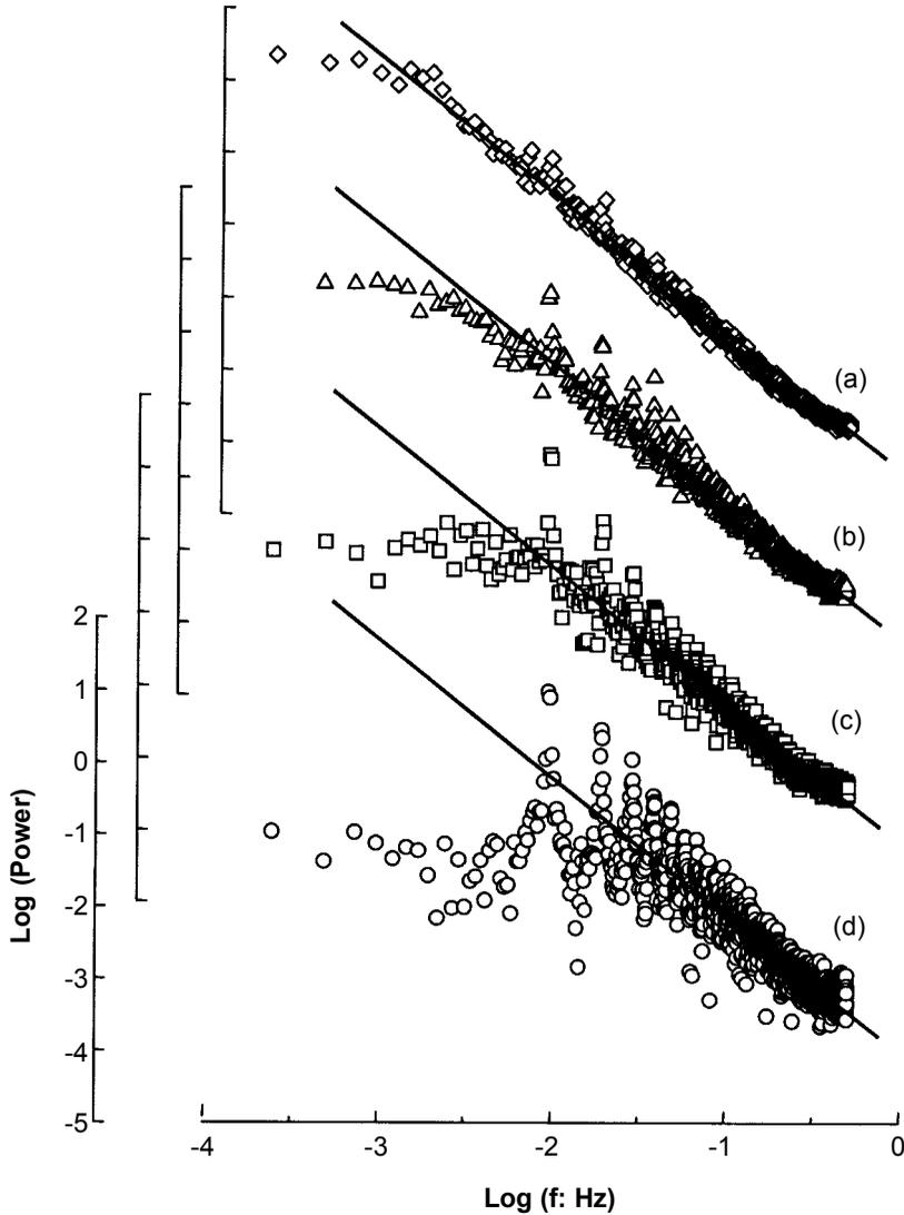
**Figure 4** Power spectra of data in Figure 3 obtained using fast fourier transformation [(a) public vehicles = 10, (b) public vehicles = 50, (c) public vehicles = 100, and (d) public vehicles = 500]. The total number of vehicles was fixed at 2000, the iteration step at  $10^4$ , the stopping time at 100 steps,  $p_c = 0.2$ , and  $\gamma = 0.1$ . Straight lines are fitted for those curves
