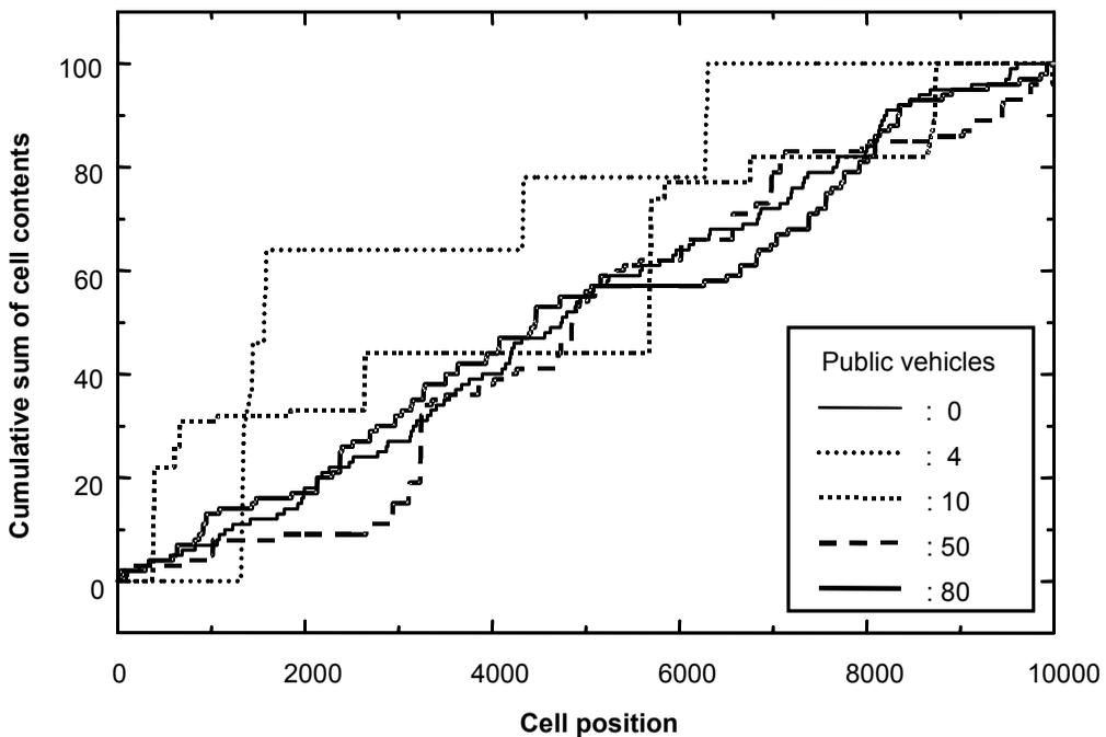
**Figure 2** Cumulative sum of cell contents as a function of cell position simulated using Equations (4) and (5). Data were obtained for different number of the public vehicles. The total number of vehicles was fixed at 100, the iteration step at  $10^4$ , the stopping time at 100 steps, and  $p_c = 0.2$ , and  $\gamma = 0.1$
