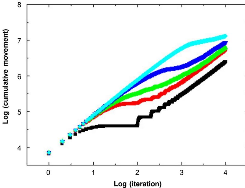
**Figure 5** Cumulative movement as function of iteration time both in logarithmic scales at different number of public vehicles (top to bottom: 2, 10, 50, 100, and 500). The total number of vehicles was fixed at  $10^4$ , the stopping time at 100 steps,  $p_c = 0.2$ , and  $\gamma = 0.1$
