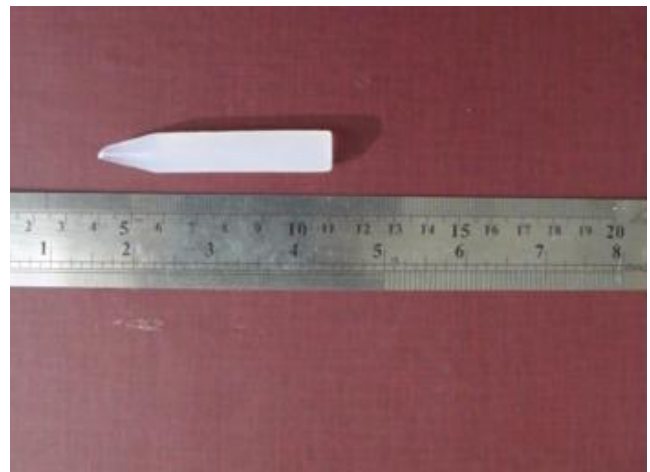
Figure 5 Monolithic crack-free aerogel
