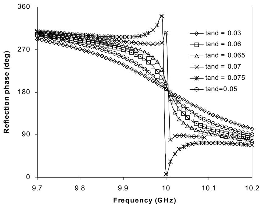
**Figure 3** Phase curve variation of the periodic array with different dissipation factors
