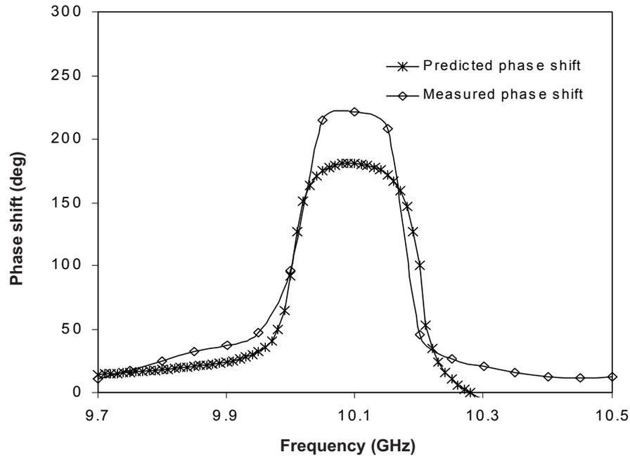
**Figure 7** Measured and simulated phase shift curve of the periodic array
