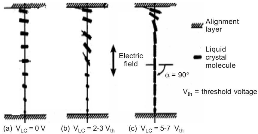
**Figure 1** Change in the position of the LC molecules with increasing voltage [8]
