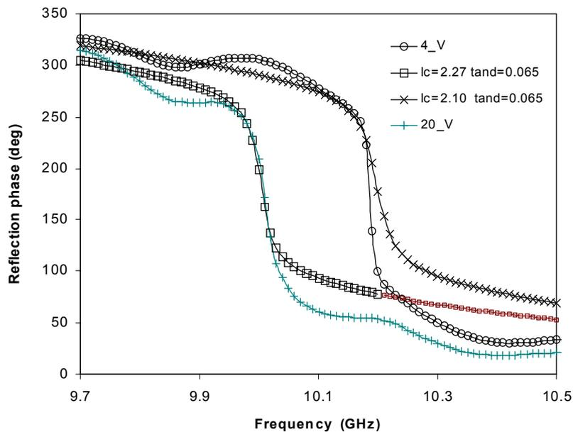
**Figure 6** Measured and simulated phase response of the periodic array
