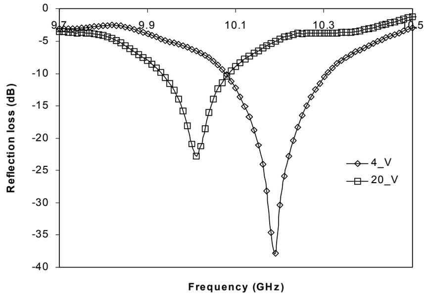
**Figure 5** Measured reflection loss at two different voltage states
