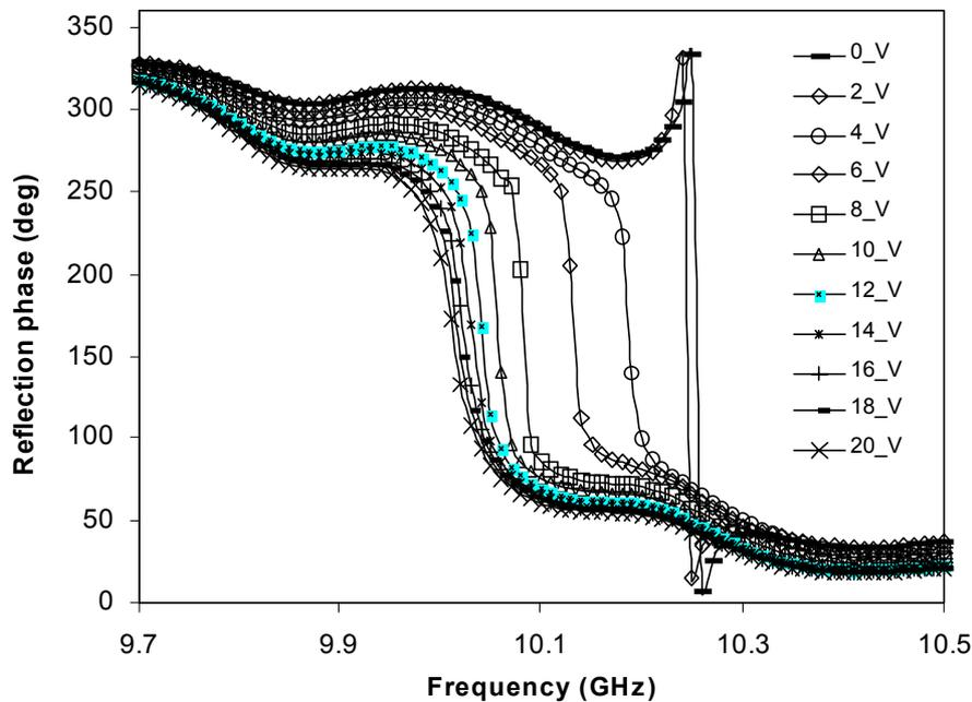
**Figure 4** Measured phase response of the periodic array with applied dc voltage
