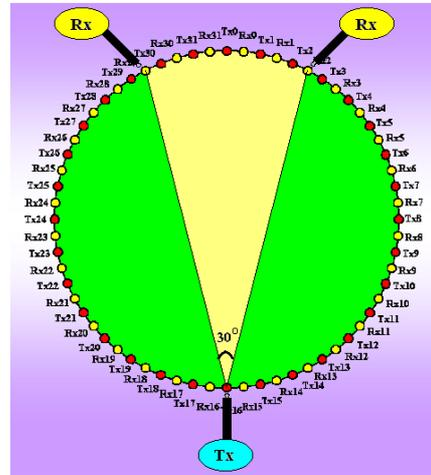
**Figure 9** Determining emission angle
