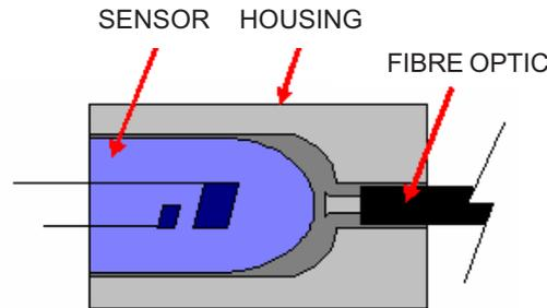
**Figure 8** Coupling between sensor and fibre optic
