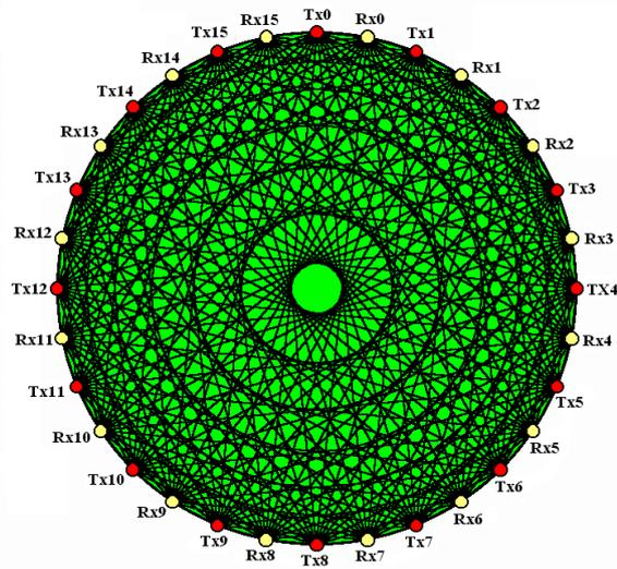
**Figure 2** Sensor configuration in switch-mode fan beam projection method
