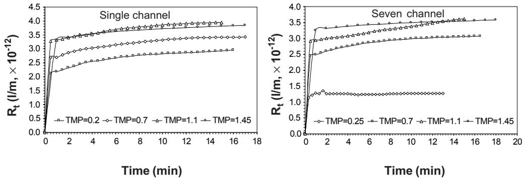
Figure 6 Plot of total membrane resistance versus time at 30°C and at various pressures
