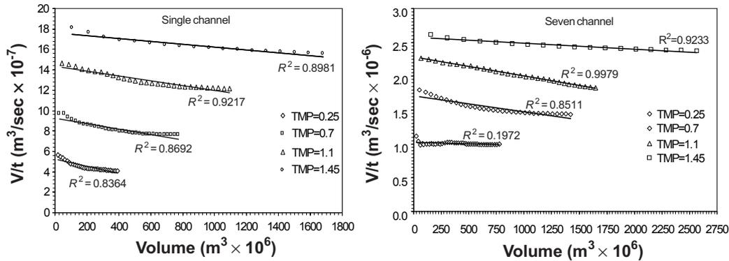
**Figure 10** Plot of filtration data for gasification effluent according to Hermia complete pore blocking model (CPBM) at varying TMP
