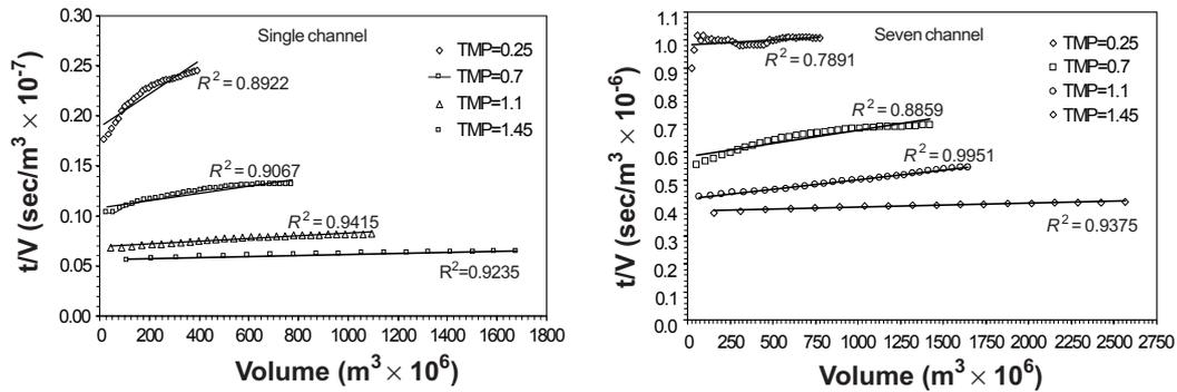
**Figure 8** Plot of filtration data for gasification effluent according to Hermia cake formation model (CFM) varying TMP
