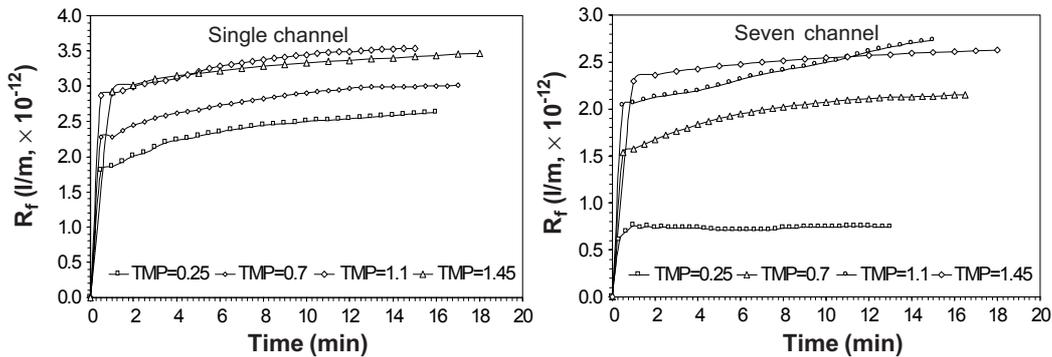
Figure 7 Plot of membrane fouling layer resistance versus time at 30°C and at various pressures
