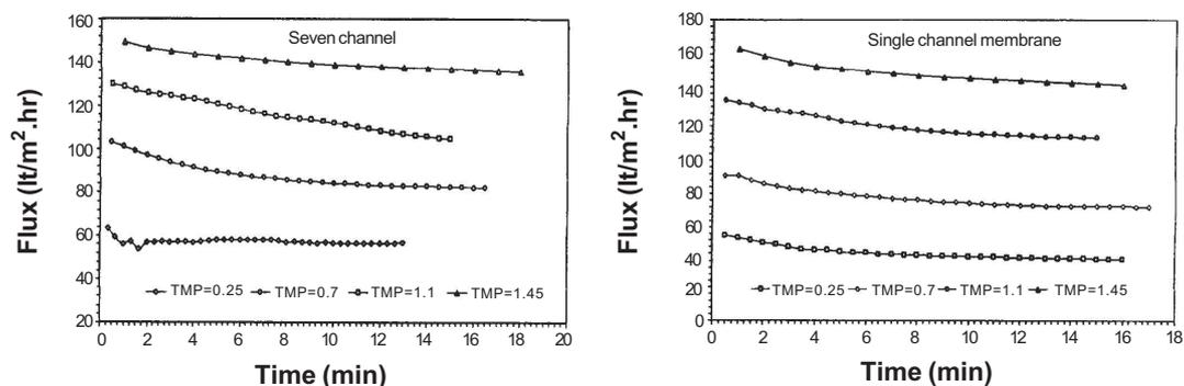
Figure 5 Plot of flux with respect to time for various TMP at 30°C
