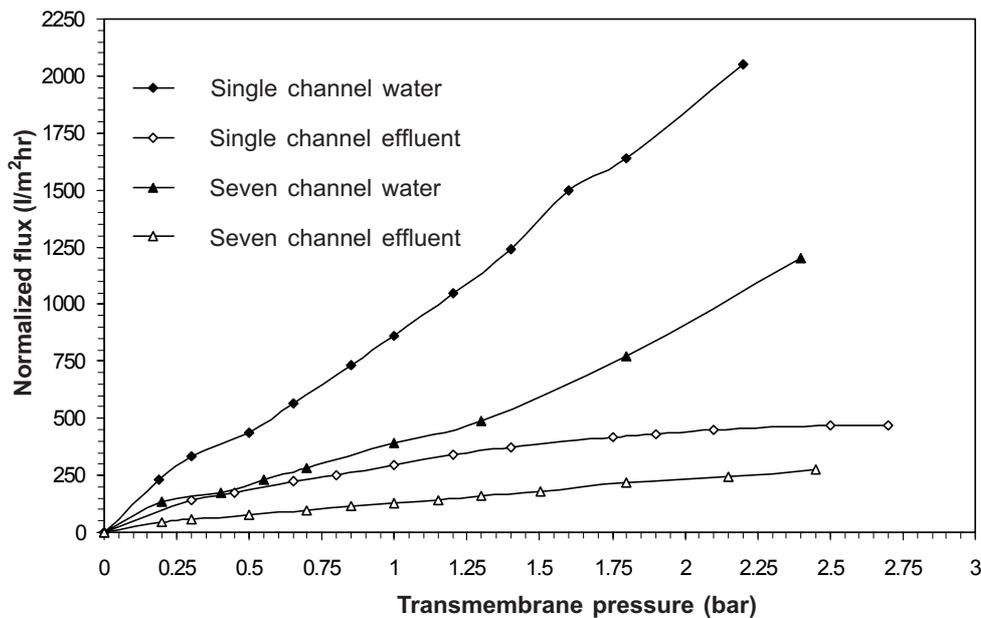
**Figure 2** Effect of transmembrane pressure on flux, at 30°C, for membranes with pore size of 1.2 μm
