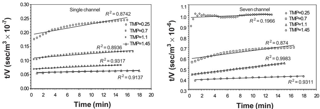
**Figure 9** Plot of filtration data for gasification effluent according to Hermia standard blocking model (SBM) at varying TMP
