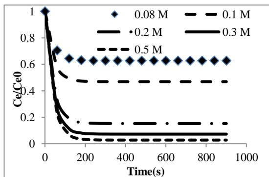
**Figure 4** Varies carrier concentration on effect of kraft lignin extraction. [Condition: Concentration of feed phase = 4600ppm, treat ratio = 0.2, pH = 3.6]
