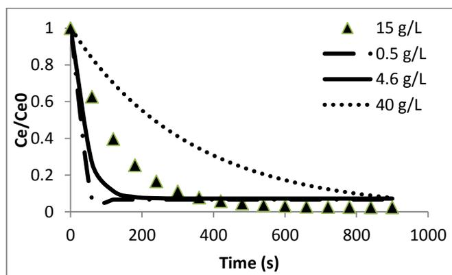
**Figure 5** Effect of initial concentration of kraft lignin at external phase on extraction performance. [Condition: Carrier concentration = 0.3M, treat ratio = 0.2, pH = 3.6]
