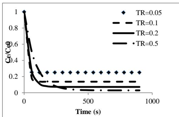
**Figure 3** Varies treat ratio on effect of kraft lignin extraction. [Condition: Concentration of feed phase = 4600ppm, Carrier concentration = 0.3M, pH = 3.6]
