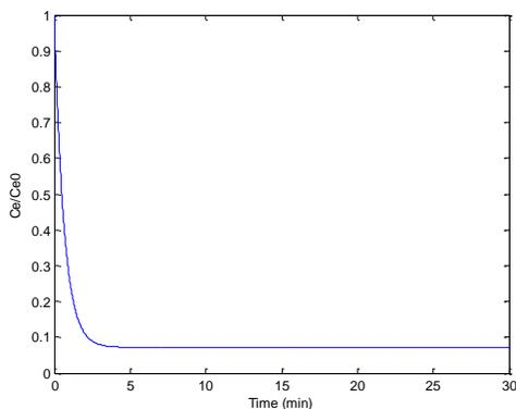
Figure 1 Concentration of solute at external phase for 30mins. [Condition: Concentration of feed phase = 4600ppm, carrier concentration = 0.3M, treat ratio = 0.2, pH = 3.6]
