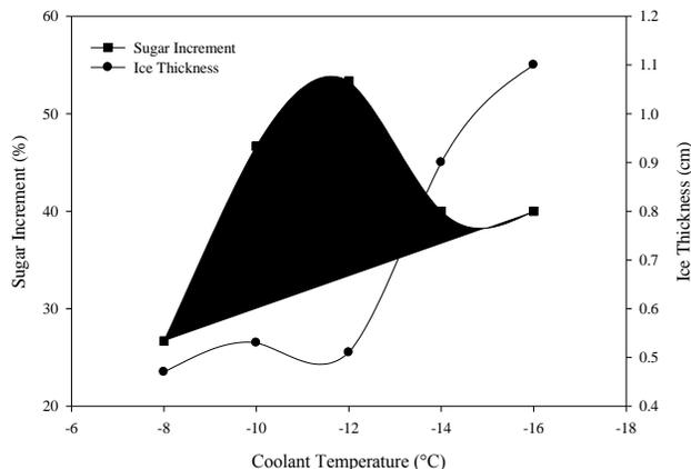
**Figure 8** Effect of coolant temperature on sugar concentration
