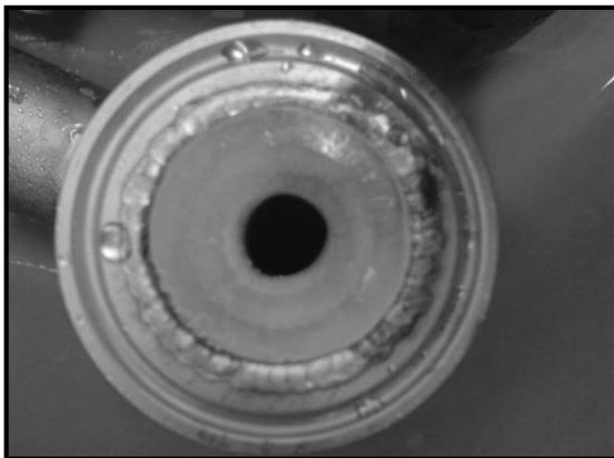
Figure 3 A close-up of the ice layer formed
