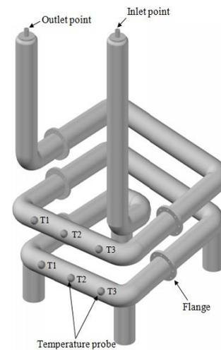
Figure 1 Stainless steel crystallizer
