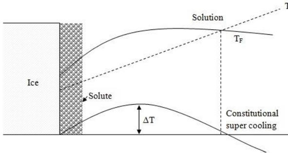
Figure 5 Constitutional supercooling during freezing process of solutions [17]
