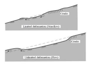
Figure 4 Flow and non-flow deformation of sandy soil<sup>2</sup>
