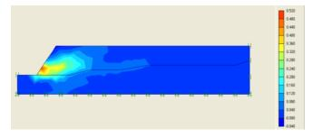
Figure 7 Strain in the slope when soil is dry<sup>1</sup>
