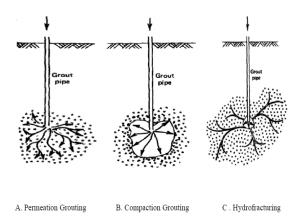
Figure 5 Types of grouting system<sup>6</sup>
