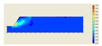
Figure 9 Incremental strains after heavy rain<sup>1</sup>
