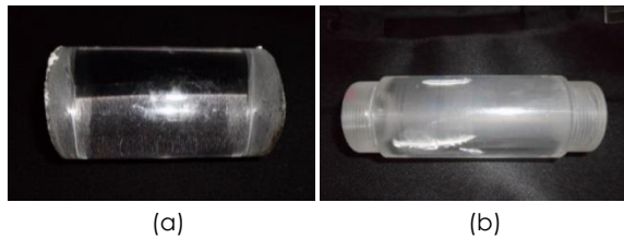
Figure 6 Picture of mixing chamber (a) as raw perspex and (b) after completion of machining
