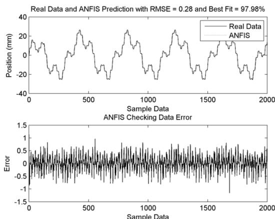
Figure 12 2 Inputs 4 membership function model simulation
