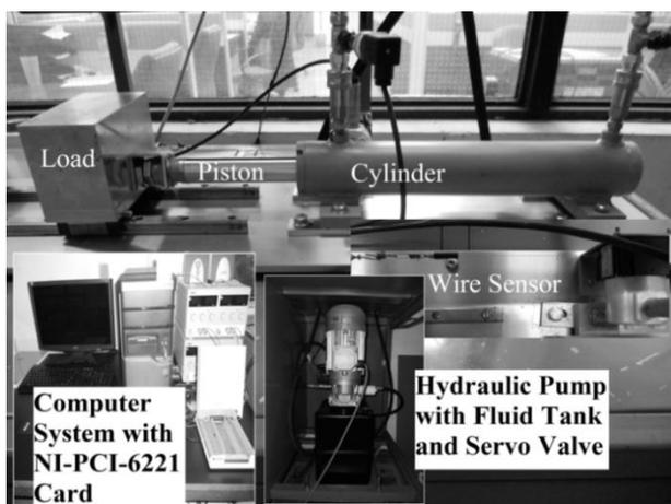
Figure 1 Experiment setup
