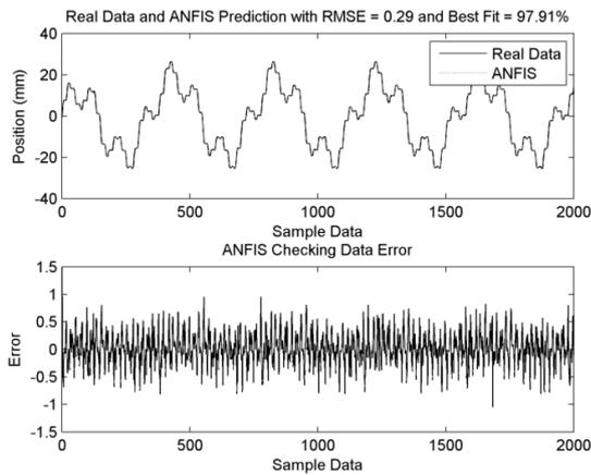
Figure 10 2 Inputs 3 membership function model simulation
