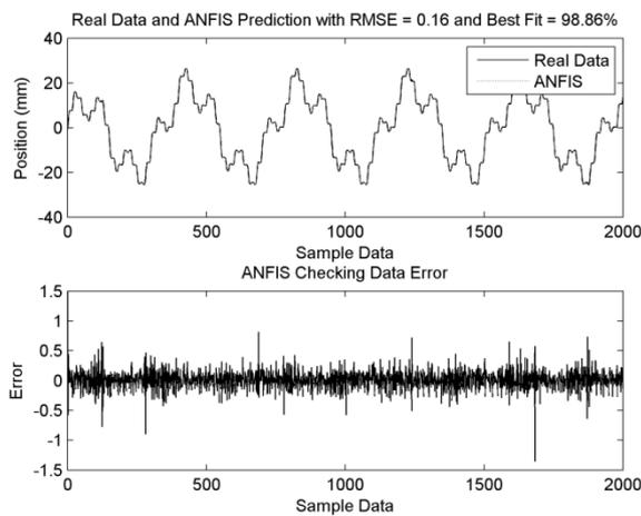
Figure 8 3 Inputs model simulation
