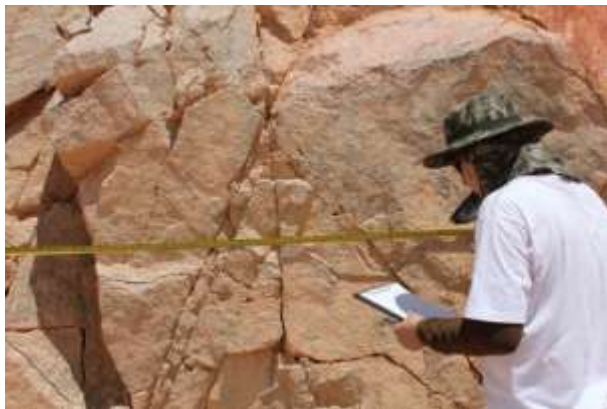
Figure 3 Example of scanline sampling for joint survey
