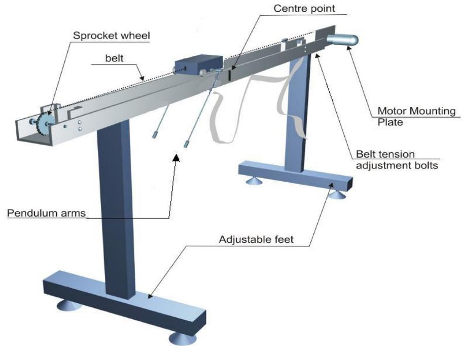
Figure 15 Real inverted pendulum used in this work [11]
