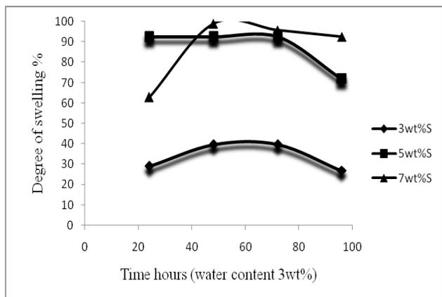
**Figure 4** Effect of time and sago content on the degree of swelling of blended membrane
