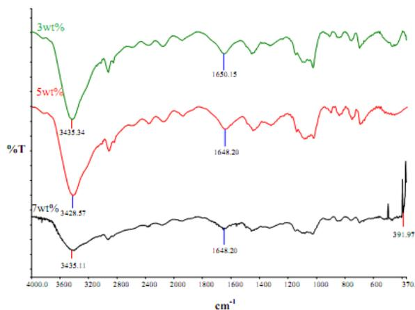
Figure 2 FTIR spectra of blended sago membrane and blended ration
