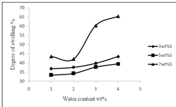
**Figure 3** Effect of degree of swelling on the blended ratio membranes (3wt%, 5wt% and 7wt% of sago)
