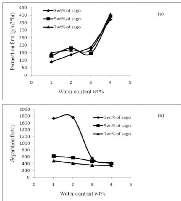
Figure 6a, b showed the effect of water content in the feed on the permeation flux and separation factor
