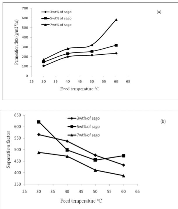
**Figure 5 a, b** showed the effect of feed temperature on the permeation flux and separation factor
