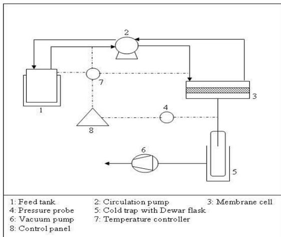
Figure 1 Schematic diagram of pervaporation process
