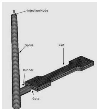
**Figure 1** The design of the tensile bar and feeding system
