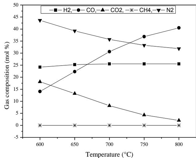
**Figure 1** Effect of temperature on product gas composition
