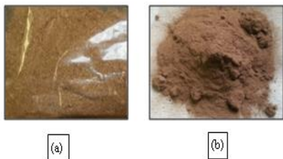
Figure 1 Physical appearance of oil palm mesocarp fiber (a) before extraction, and (b) residue
