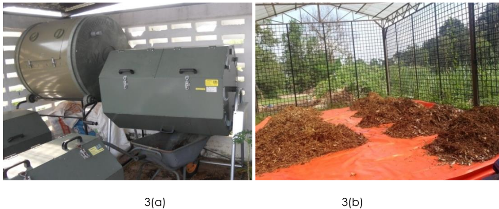
Figure 3 Composting technique that has been used in UKM; (a) rotary drum (in – vessel technique) (b) the turned windrow
