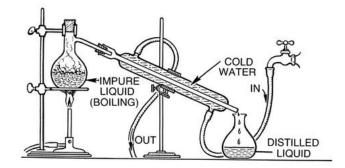
Figure 2 A typical distillation process [8]
