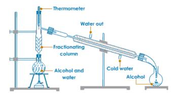
Figure 3 Fractional distillation process [9]
