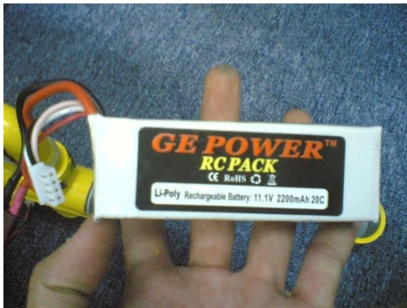
Figure 11 ROV 12 volts 220 mAh Lithium Polymer battery
