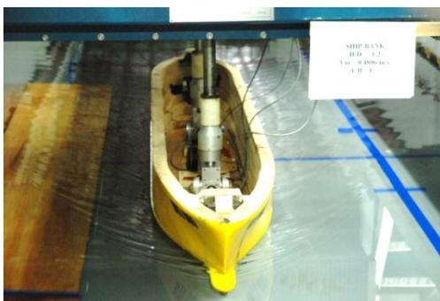
Figure 6 Ship model in testing situation with bank-shallow water
