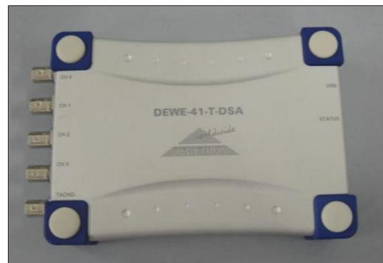
**Figure 16** Data acquisition system
