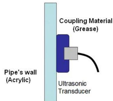
Figure 2 Acoustic coupling placement for ultrasound transmission
