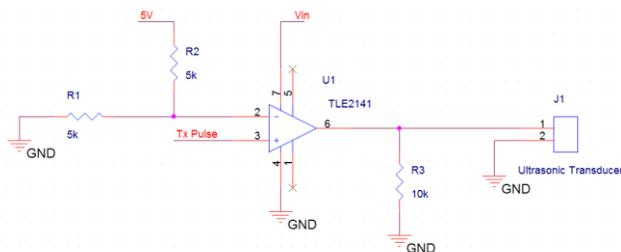
Figure 4 Pulse generator circuit schematic
