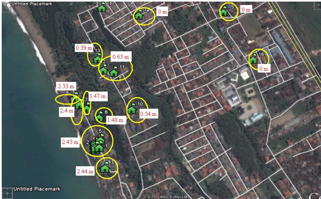
Figure 3 Map of tsunami inundation against the buildings in Parupuk Tabing
