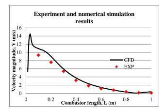
Figure 3 Velocity magnitude profile along combustor
