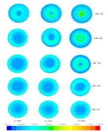
**Figure 6** Contour of axial velocity of various swirl number and x/D at z-plane
