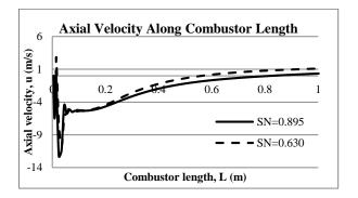
Figure 5 Comparison of axial velocity along combustor length
