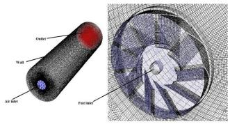
Figure 1 The mesh modeling of unconfined burner including the axial swirler
