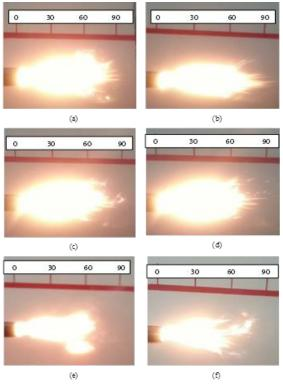
Figure 5 Flame length at equivalent ratio 1
