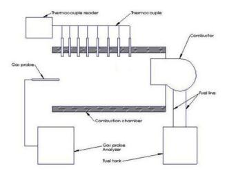
Figure 1 Schematic of experimental set-up for combustion test
