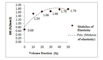
**Figure 8** Graph showing the relationship between the modulus of elasticity (E) with a ratio of volume fraction variation
