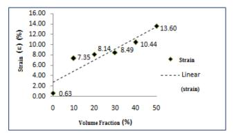
Figure 7 Graph showing the relationship between strain with a ratio of volume fraction variation
