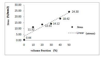
Figure 6 Graph showing the relationship between stress with a ratio of volume fraction variation
