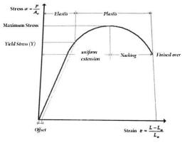
Figure 2 Graph stress versus strain
