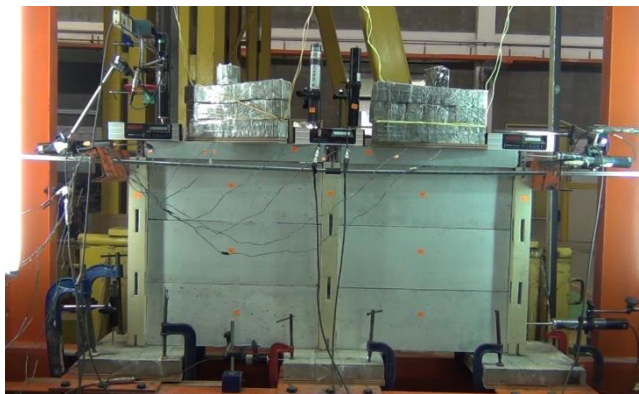
Figure 7 Cycle 1: (a) load - horizontal displacement relationship; (b) sketch of front view crack pattern; (c) sketch of back view crack pattern; (d) photograph
