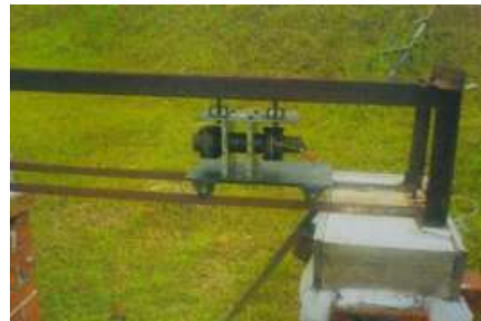
Figure 21 A rocket motor was on a rail for dynamic test 19
