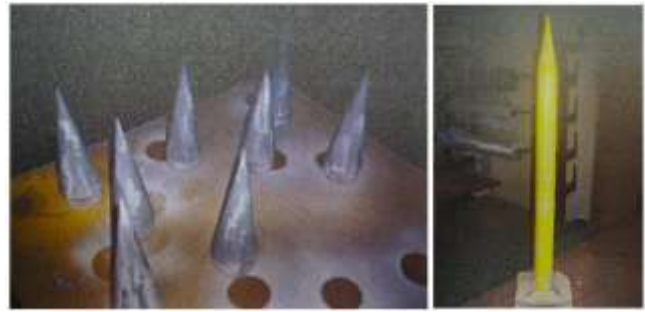
Figure 26 Patty sealing process on rocket body (left) and assembly of rocket body (right) 25
