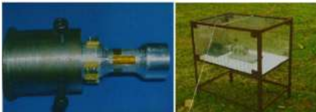
Figure 19 UTM-designed dumbbell shaped load cell (left) and load cell assembly in the static test station (right) 18
