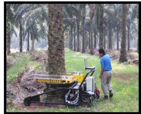
Figure 2 GammaScorpion is being used to scan the trunk of palm oil [6]
