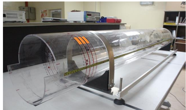
Figure 8 Three different perimeters setup on the Perspex pipeline system
