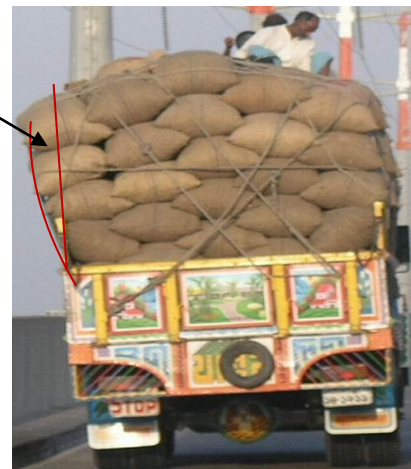
Figure 3 Forces and reactions of a heavy truck in rigid vehicle model (left) and bulging/shifting of load on a truck (right)
