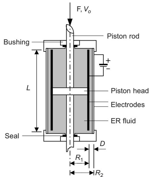
**Figure 2** Flow mode ER damper
