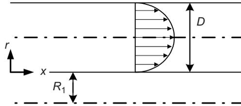
**Figure 4** Newtonian fluid velocity profile
