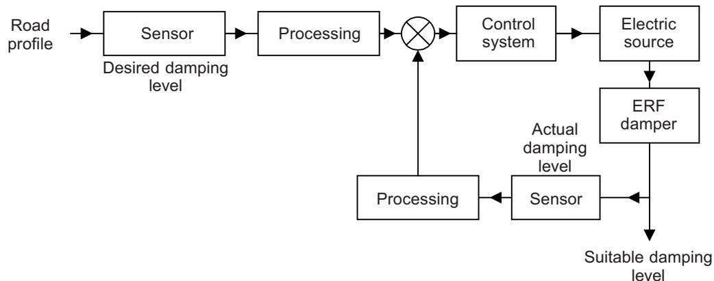
**Figure 1** Schematic diagram of an intelligent ER suspension system [1]
