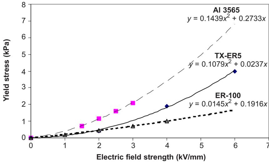
**Figure 6** Effect of electric field strength to the  $\tau_y$
