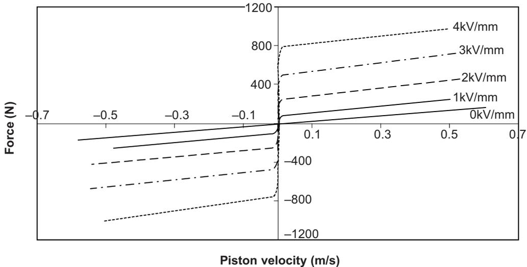
**Figure 8** Force versus velocity diagram for nominal damper filled up with Al 3565
