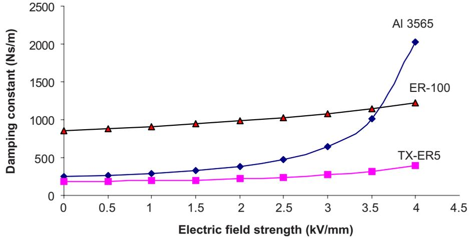
**Figure 7** Relationship between electric field strength to the damping constant for nominal damper filled up with particular fluid
