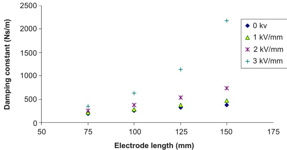
**Figure 10** Effect of electrode length variation to the damping constant for various electric field strength
