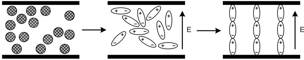
**Figure 3** Schematic illustrations of the ER particles before and after application of an electric field. The two parallel dark lines stand for two electrodes [5]
