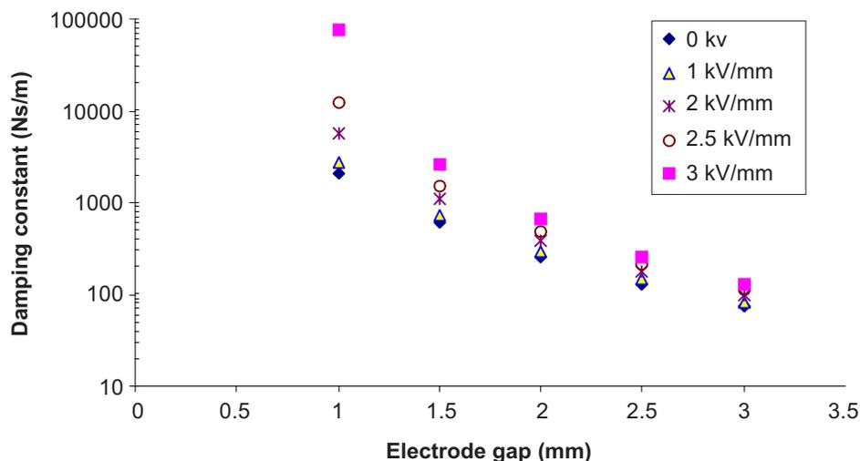
**Figure 9** Effect of electrode gap variation to the damping constant for various electric field strength
