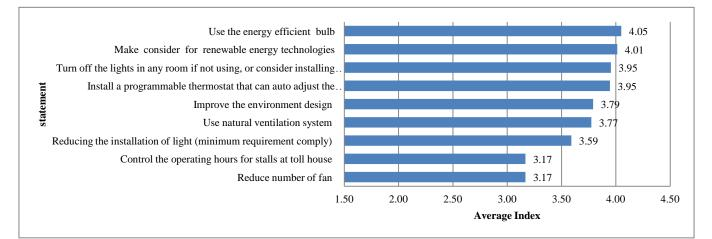
Figure 4 Potential action to reduce energy consumption in toll hous
