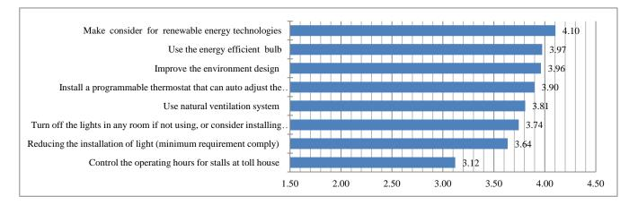
Figure 5 Potential action to reduce energy consumption in toll booth
