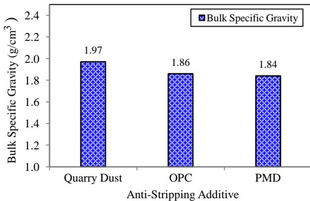
Figure 1 Comparison of bulk specific gravity for compacted mixes
