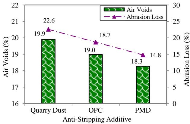
Figure 3 Air voids effect on dry abrasion loss
