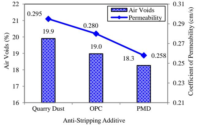
Figure 4 Result of air voids on coefficient of permeability
