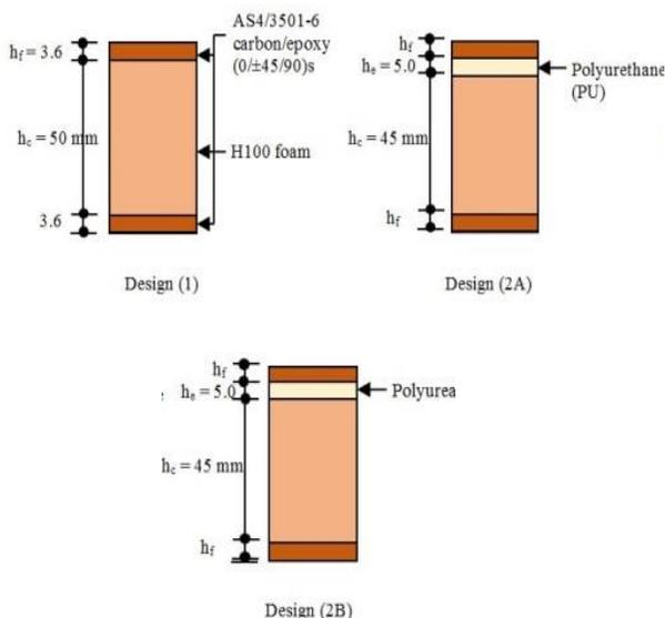
**Figure 4** Cross sections of conventional and modified designs of sandwich panels, as shown in Bahei-El- Din and Dvorak [36]
