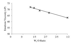
Figure 6 Plot of emulsion viscosity against W1/O ratio
