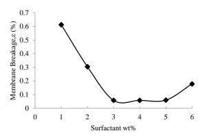
Figure 3 Effect of surfactant concentration on membrane breakage
