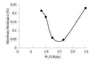
Figure 5 Effect of W1/O ratio on membrane breakage
