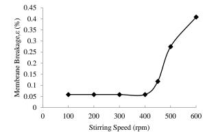
Figure 9 Effect of stirring speed on membrane breakage
