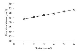
Figure 4 Plot of emulsion viscosity against surfactant concentration
