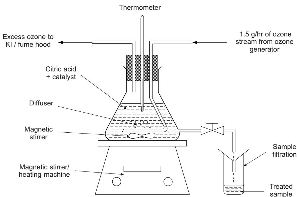
**Figure 1** Schematic diagram for the ozonation reactor
