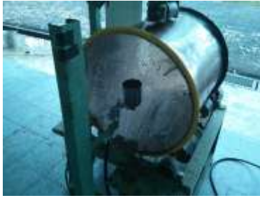
Figure 2 Mixing drum equipped with airless spray gun
