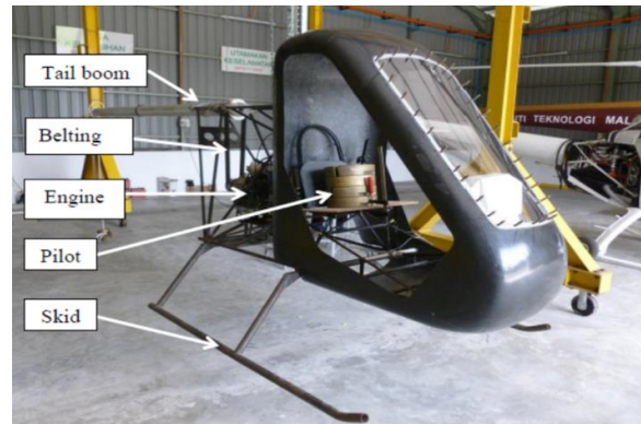
Figure 17 Loads on the chassis
