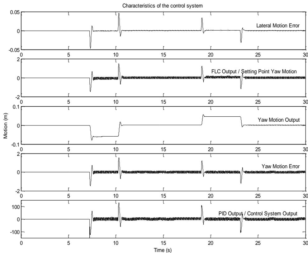
Figure 8 Characteristics of the optimal control system
