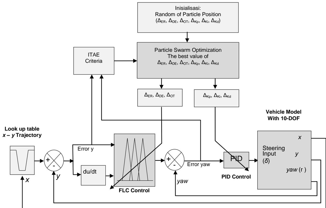
**Figure 3** The Control and Optimization Structure for active steering control on vehicle model
